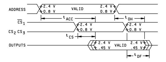
FIGURE 3. AC read timing diagram.
