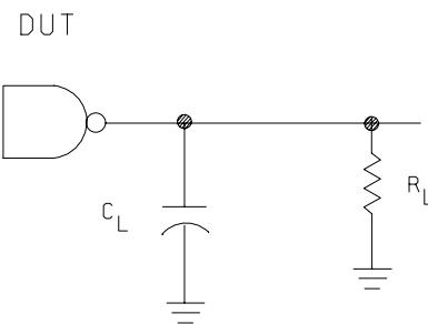
FIGURE 4. Test circuit and switching waveforms.
