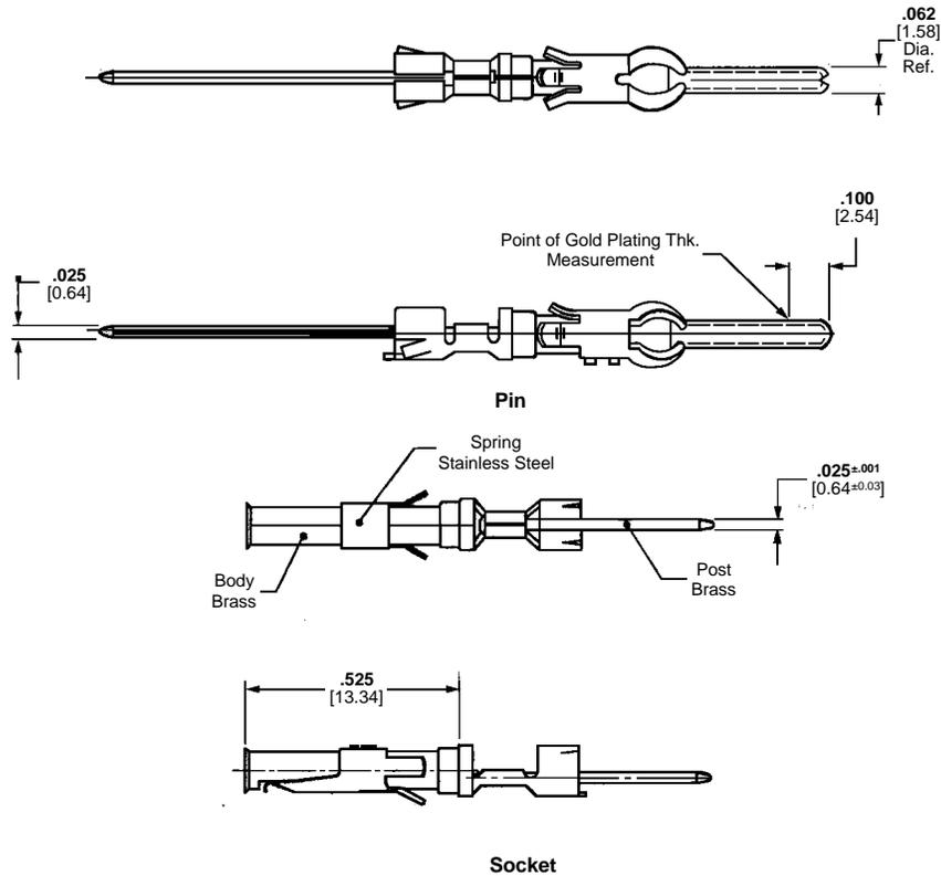
**Contact Size 16—Pin Diameter .062 [1.57] (Test Current, 13 Ampere)‡**
