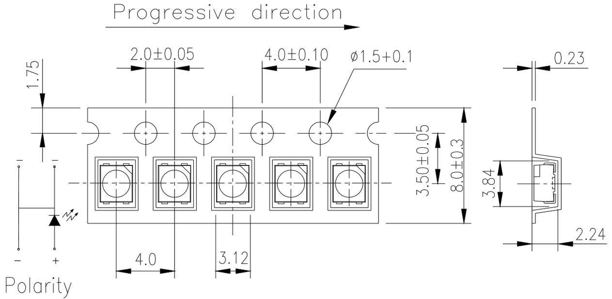
**Note:** Tolerances Unless Dimension  $\pm 0.1\text{mm}$  Unit = mm
