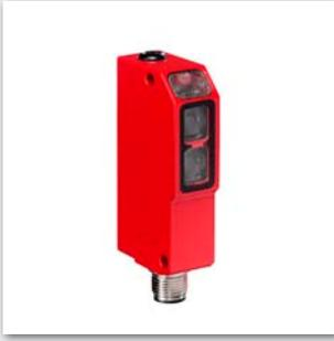
Series 95 is available as throughbeam photoelectric sensors, retro-reflective photoelectric sensors and light scanners in versions used for PET, foil and glass detection. Moreover, the sturdy housing with degree of protection IP 67 / IP 69K and the A<sup>2</sup>LS active ambient light suppression facilitate especially reliable detection, even in rough industrial environments.
