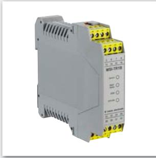
MSI-T is a safety monitoring device for the periodic testing of one-channel testable Optoelectronic Protective Devices of type 2 acc. to EN IEC 61496. Up to 6 type 2 sensors can be connected to the device in series.
