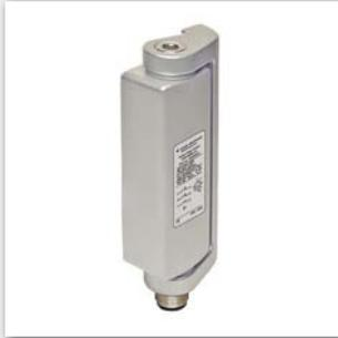
The S400 safety hinge switches unite the safety switch and door hinge functions in one component. Because external actuators are not required with this switch, it can also be used problem-free in environments with high dust concentration levels or with heavy particle loads (protection rating IP 67). By means of a repeatable setting (switching angle alignment), fault-free function is ensured even with warped or misaligned doors.
