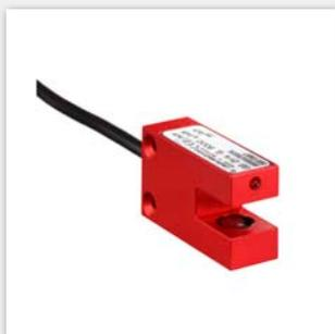
The compact forked photoelectric sensor with a mouth width of 8 mm and a switching frequency of 1000 Hz is suitable for the detection of small parts and aperture discs.
