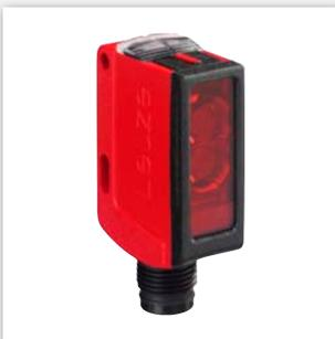
The SLSR 25B light beam safety device scores with its optimized light beam propagation (opening angle) with time-saving alignment. In combination with a safety-relevant control system (testing according to EN IEC 61496-1), it forms a category 2 contactless protective device and works with a range of up to 22 m.
