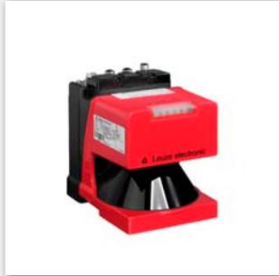
Contactless laser scanners for object detection and contour measurement. A laser measurement beam is deflected by a rotating mirror and covers an area of 190° with a radius of up to 65 m. The measurement contour is output via Ethernet or a serial interface. In addition, there are models for object detection in up to four simultaneous detection fields.
