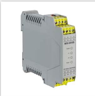
Two devices can be connected to the MSI-SR5 safety relay, either with two transistor OSSDs or by designing as a two-channel contact circuit. As a result, two sensors can be connected to a common switch-off circuit – for applications up to Performance Level PL<sub>e</sub> acc. to EN ISO 13849-1.
