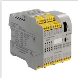
The relay monitors E-Stop buttons, two-hand controls, safety doors or safety sensors with two transistor outputs in machines and systems. With an overall width of just 67.5 mm, the device makes available 20 safe inputs, 4 signal outputs for diagnostics and 4 safe outputs (OSSDs).
