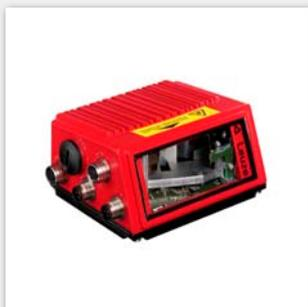
Integrated fieldbus networking is one of the key features of this series of trendsetting bar code readers. Configuration is performed via a web technology-based graphic user interface.
