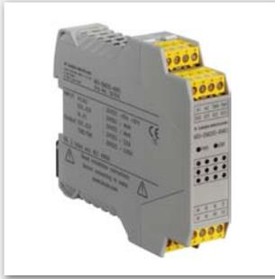
The MSI-EM extension module expands the MSI 200 programmable safety controller with 8 safe inputs and 4 freely configurable channels. These may be either safe inputs or outputs (OSSDs).
