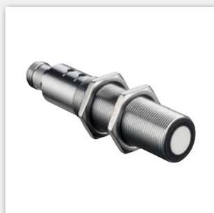
Short design, teachable and up to two independent switching outputs are the key features of this series. Also optionally available with angled head, which enables a sound outlet at 90° to the longitudinal axis of the M18 sensor. Versions available with temperature compensation and IO-Link.
