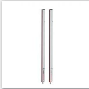
The system, which consists of transmitter and receiver, generates a monitoring field of many infrared light beams and produces a reliable switching signal as soon as objects penetrate this monitoring field. Easy installation, its small design as well as the integrated, configurable evaluation unit make the VARIO B an economical and flexible sensor solution.
