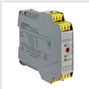
This safety relay with adjustable delay time is equipped with two release current paths which release undelayed in accordance with stop category 0. Two additional release current paths release in accordance with stop category 1 with adjustable delay time.
