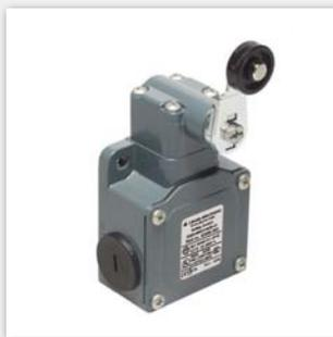
The S300 safety position switches have a metal housing in accordance with protection rating IP 67. The models equipped with various contact sets enable integration in control circuits up to category 4 in accordance with EN ISO 13849. In addition, models are available with different actuators and supports and connection options.
