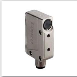
These retro-reflective photoelectric sensors in coated metal housing with glass optics were designed specially for detecting transparent PET and glass bottles, plastic foils as well as flat glass. The patented tracking process extends the cleaning interval many times over; short response times and minimal jitter ensure reliable control of fast processes. The versatile fastening options with integrated thread facilitate mounting and the models with aligned abeam optics make alignment unnecessary.
