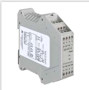
MSI-MC300 safety relays are suitable for integration of MC 300 magnetically coded sensors in control circuits up to category 4 and Performance Level PL<sub>e</sub> in accordance with EN ISO 13849-1. These kinds of magnetically coded safety systems are used, for example, to monitor movable guards such as protective doors, sliding grids or flaps.
