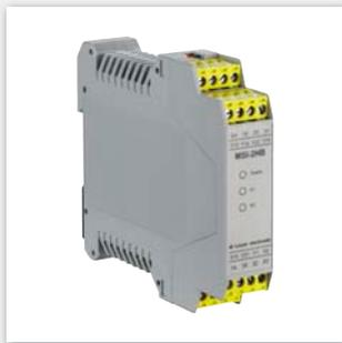
The MSI-2H is the link between two-hand command devices and the machine control. The device checks the simultaneous activation of the two, 2-channel buttons and ensures a controlled process start. The module is used everywhere that feeding-in is not automatic, but rather has to be performed manually by people.
