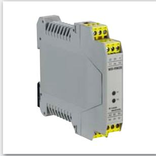
With the MSI-RM2 relay module, a compact and – at the same time – economical solution is available in combination with safety sensors for applications up to Performance Level PL<sub>e</sub>. The relay module, only 17.5 mm wide, has two potential-free make contact circuits with a response time of only 10 ms.
