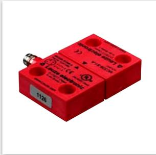
The MC3x coded magnetic sensor contains specially combined reed contacts that are contactlessly activated by the coded magnetic field of the actuator. With their cast housing, the extremely tamperproof switches are suitable for demanding applications in dusty or humid environments.
