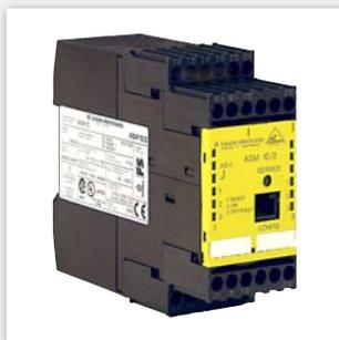
The ASM1 AS-i safety monitor is the core component of the AS-Interface Safety at Work system. Using configuration software, it monitors the safety-related network devices that are assigned to it, e. g., command devices, multiple light beam safety devices and safety switches.
