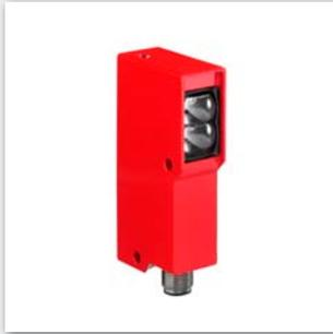
The Series 92 Ex sensors are available as reflection light scanners, retro-reflective photoelectric sensors or throughbeam photoelectric sensors and reliably detect objects at distances of 300 mm up to 12 m. The intrinsically safe sensors transmit switching signals to the VS 403 isolated switching amplifier by way of the NAMUR interface. The temperature class for explosive gas areas is T6; for explosive dust areas it is 80 °C.
