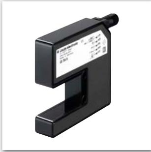
With mouth widths of 27 or 100 mm, this forking photoelectric sensor delivers accurate measurement results over a 25 mm long measurement range thanks to its CCD line. Depending on the configuration, it is possible to measure transparent edges, the diameters of wires, threads and much more.
