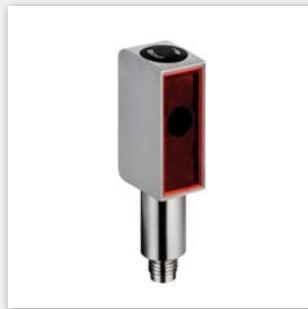
These sensors were specially designed for sensitive hygiene applications, e. g., in the pharmaceutical, cosmetic and food industries. Their housing is consistently designed for preventing bacterial carry-overs with its scratch resistant and non-diffusive plastic screen. The unique fastening concept, which consists of a mounting trunion with 12 mm diameter and G6 fit, ensures a gas-tight connection between sensor and machine.
