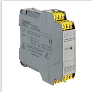
The MSI-CM safety relay is used as a contact extension module in accordance with DIN EN 60204-1/VDE 0113 Part 1 for contact extension for E-Stop relays and two-hand control units. Depending on the wiring and proper integration of the feedback path, a Performance Level PL e in accordance with EN ISO 13849-1 is achieved.
