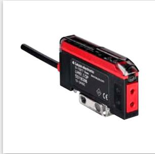
The series satisfies all basic requirements: 20-turn potentiometer for high-resolution sensitivity adjustments, two switches for light/dark switching and for selecting between larger range or higher switching frequency.
