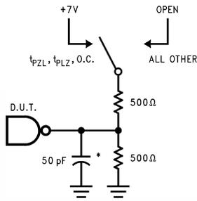
\*Includes jig and probe capacitance
