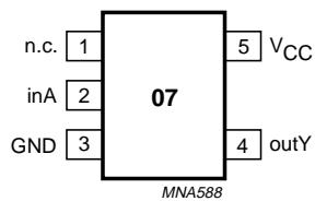
Fig.1 Pin configuration.
