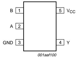
**Fig 4. Pin configuration**
