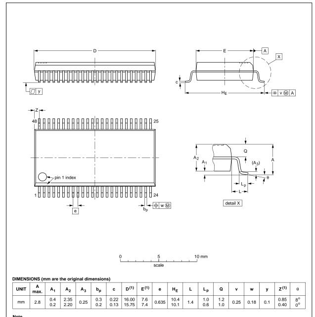
1. Plastic or metal protrusions of 0.25 mm maximum per side are not included.
