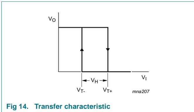
**Fig 14. Transfer characteristic**
