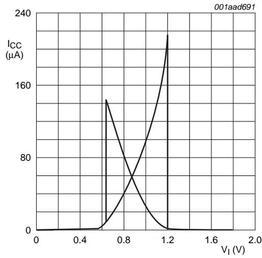
Fig 16. Typical transfer characteristics;  $V_{CC} = 1.8 V$
