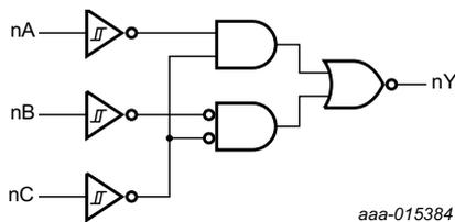
Fig 1. Logic symbol (one gate)
