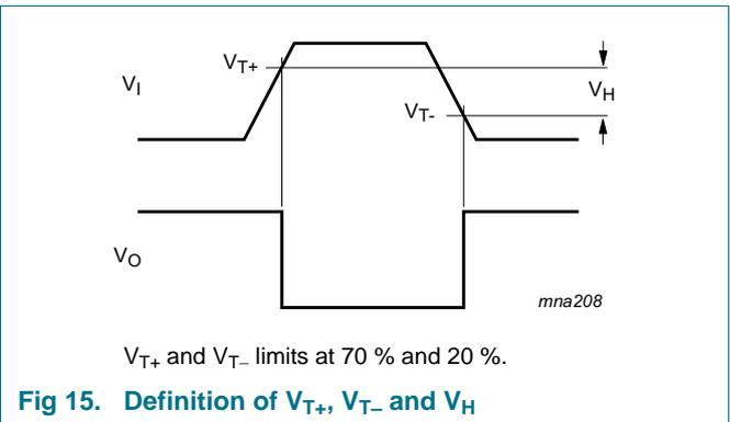
**Fig 15. Definition of V<sub>T+</sub>, V<sub>T-</sub> and V<sub>H</sub>**
