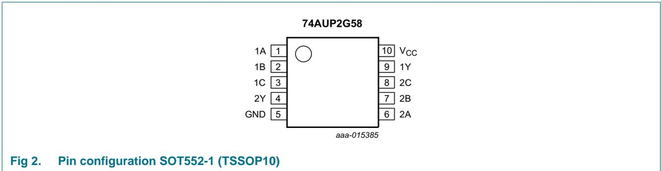
**Fig 2. Pin configuration SOT552-1 (TSSOP10)**
