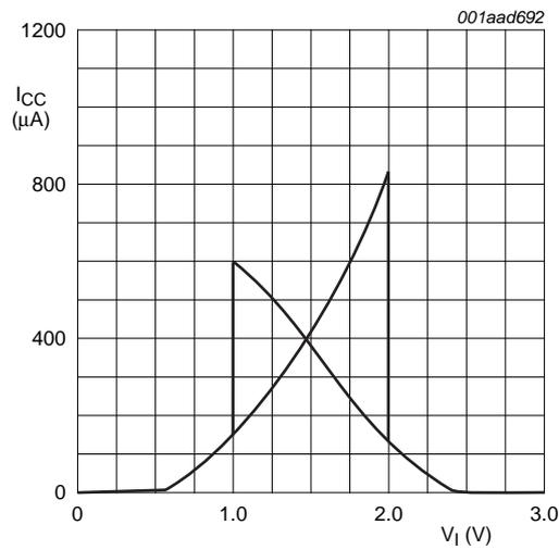
Fig 17. Typical transfer characteristics;  $V_{CC} = 3.0 V$
