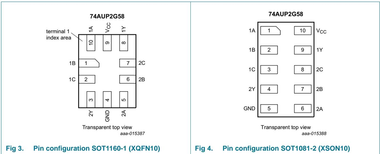
**Fig 3. Pin configuration SOT1160-1 (XQFN10)**
