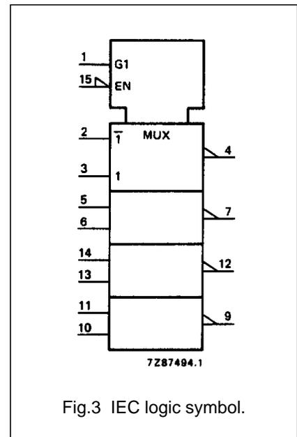
Quad 2-input multiplexer; inverting
