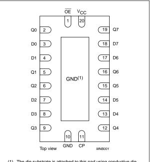
(1) The die substrate is attached to this pad using conductive die attach material. It can not be used as a supply pin or input.
