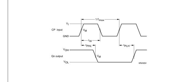
$V_M = 1.5 \text{ V at } V_{CC} \ge 2.7 \text{ V}.$
