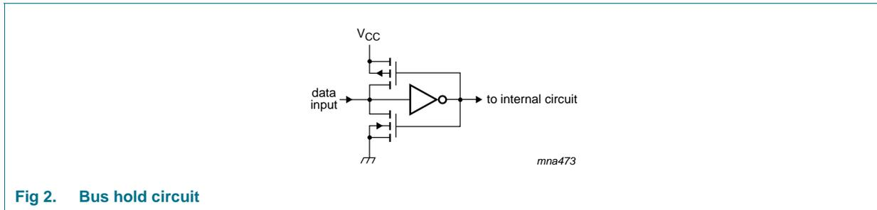
Fig 2. Bus hold circuit
