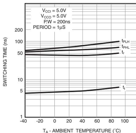
**Figure 9. 74OL6010/11 Switching Times vs. Ambient Temperature**
