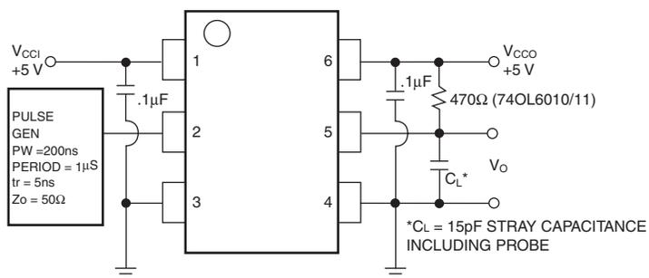
**Figure 16. Common Mode Rejection Test Circuit**
