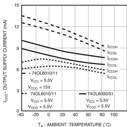
Figure 4. Output Current vs. Ambient Temperature
