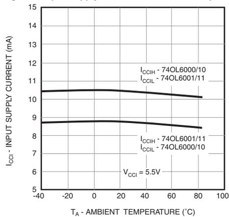
Figure 3. Output Supply Current vs. Ambient Temperature
