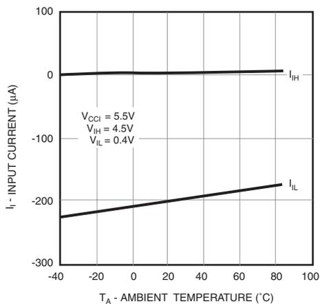
Figure 2. Input Supply Current vs. Ambient Temperature
