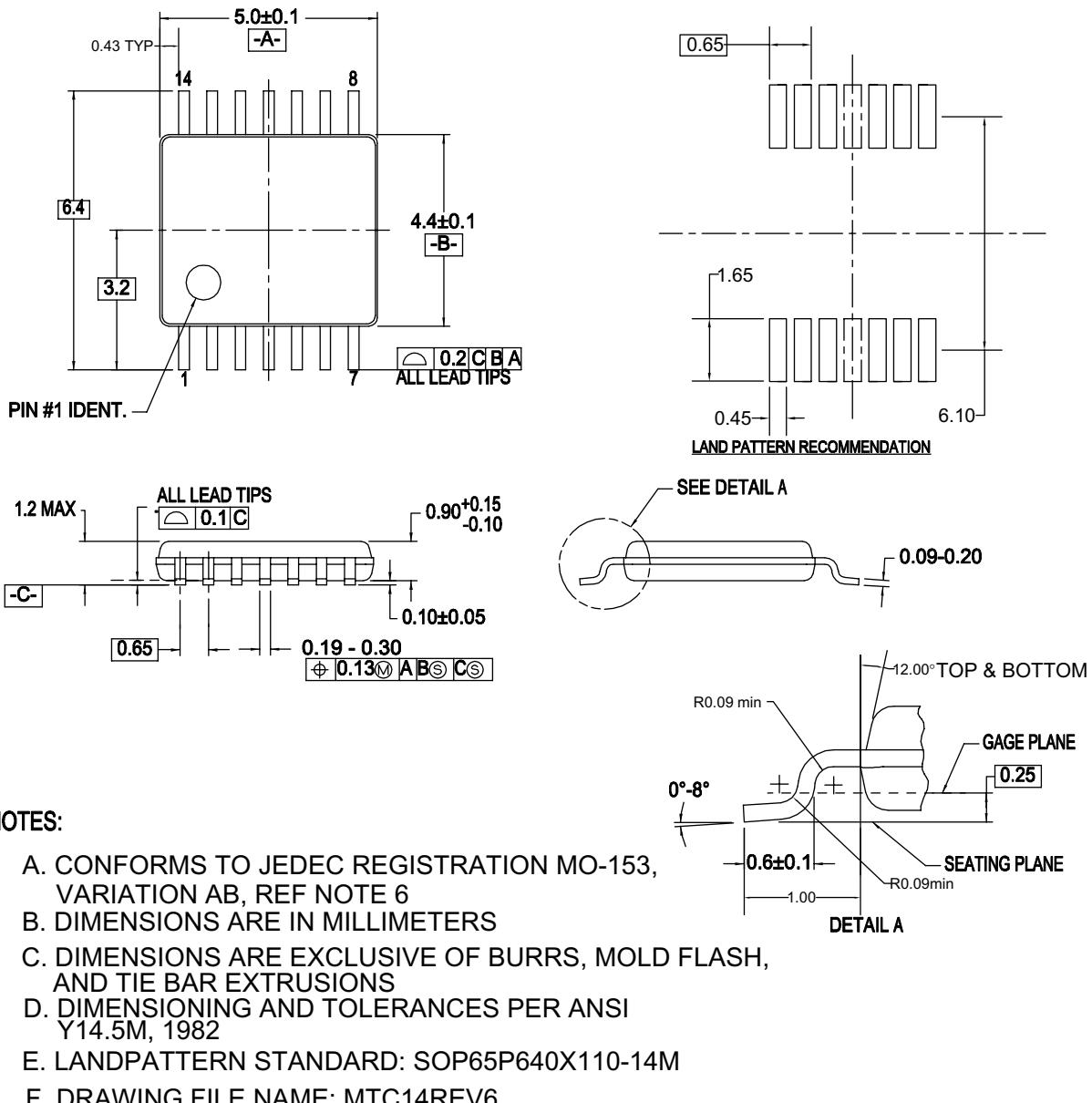
Figure 3. 14-Lead Thin Shrink Small Outline Package (TSSOP), JEDEC MO-153, 4.4mm Wide
