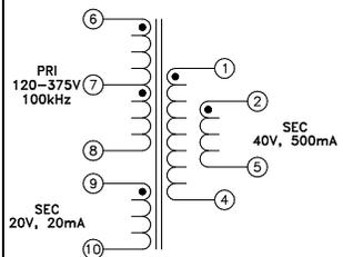
Customer to tie terminals 1+2 and 4+5 internally on the pc board.
