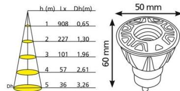
230 led BULB – GU10 warm white color (2900K°) or white color (5000K°), with COB LED (Chips On Board) high power brightness for burn life about 30000 hours. With 38° beam lighting and 600 lumens it can replace conventional halogen lam.
