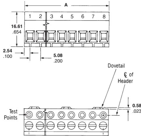
**5.08 mm Flush-Mount Plug-In Connectors with Cage Clamp Series B51C8 (Mate with Series B71N8 Pin Headers)**
