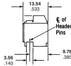
**5 mm Flush-Mount Plug-In Connectors with Cage Clamp Series B51C4 (Mate with Series B71N4 Pin Headers)**
