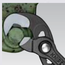
Working on tight nuts with rounded edges
