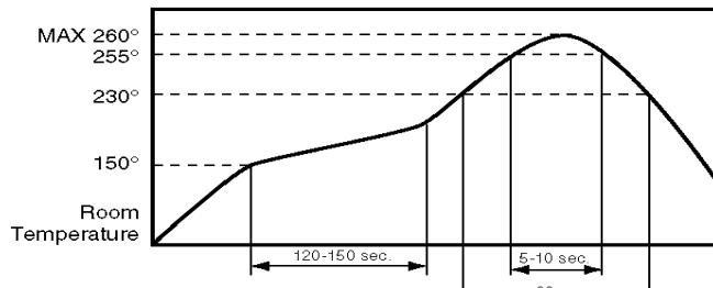
WAVE SOLDERING: 260°C maximum solder temperature for 5 seconds max.
