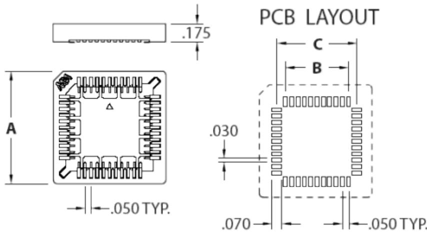
FOR PRINTED CIRCUIT DRILLING PATTERNS
