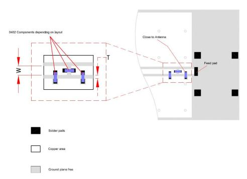
The antenna feed pad and the antenna ground pad are indicated in the drawing above. Additional pads are for mechanical attachment only and should not be grounded.
