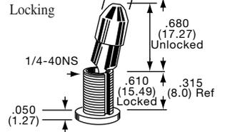
No bushing option needed for "K" or "K1" "K" locking levers are used to prevent accidental switching and must be lifted up prior to actuation. Standard nickel finish.
