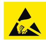
Caution! ESD sensitive device. Precautions should be used when handling the device in order to prevent permanent damage.
