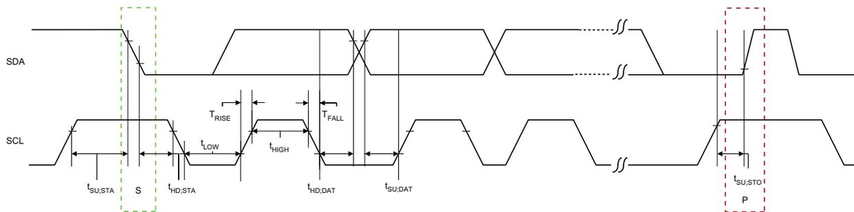
**Figure 2-47 • I<sup>2</sup>C Timing Parameter Definition**
