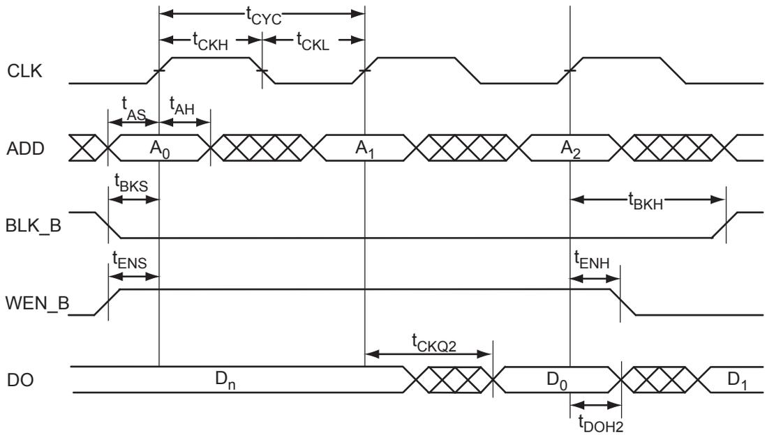
Figure 2-31 • RAM Read for Pipelined Output
