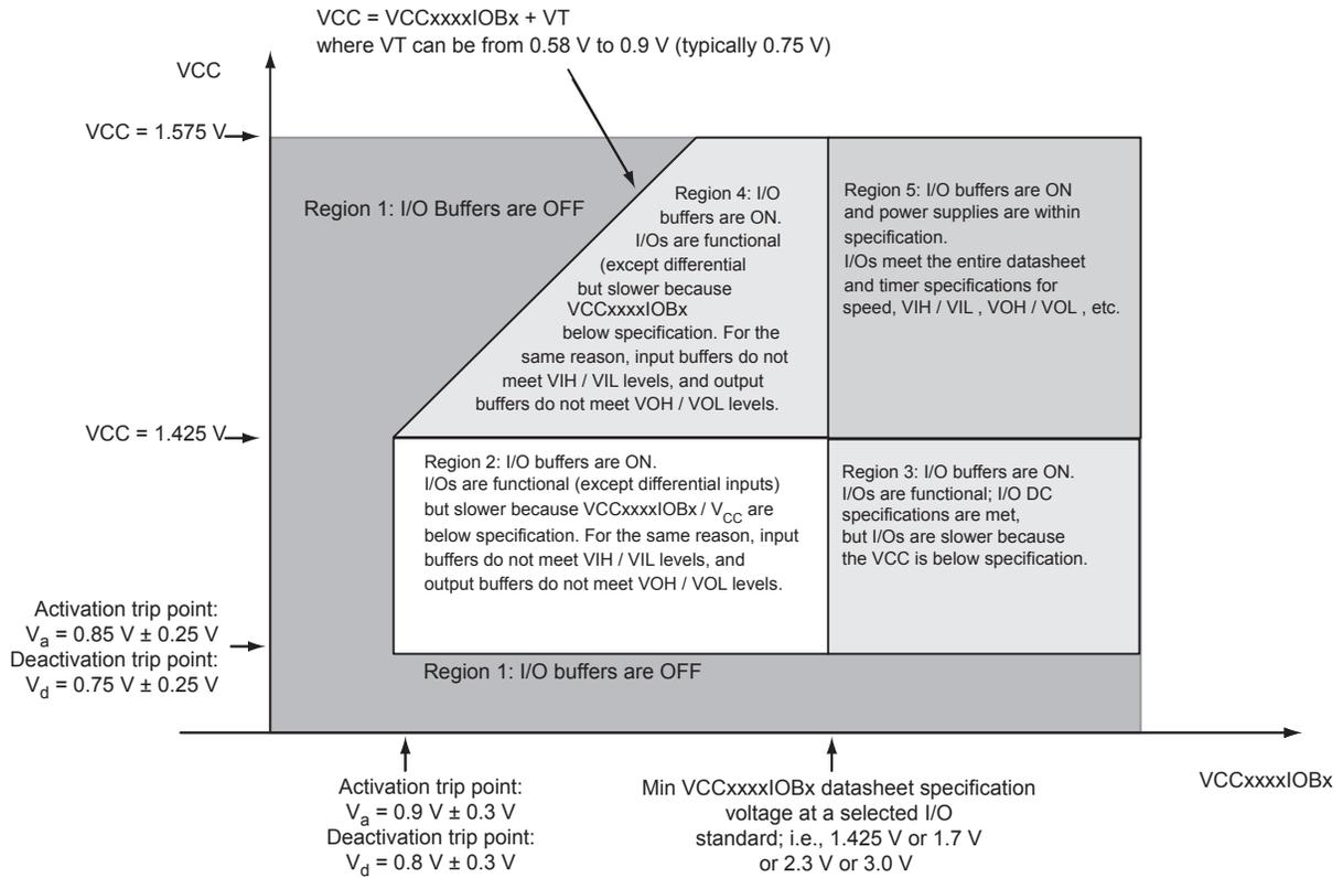
**Figure 2-1 • I/O State as a Function of  $V_{CCxxxxIOBx}$  and  $V_{CC}$  Voltage Levels**
