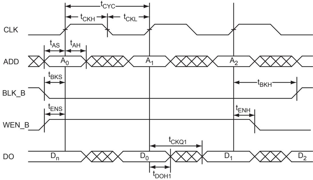
Figure 2-30 • RAM Read for Pass-Through Output
