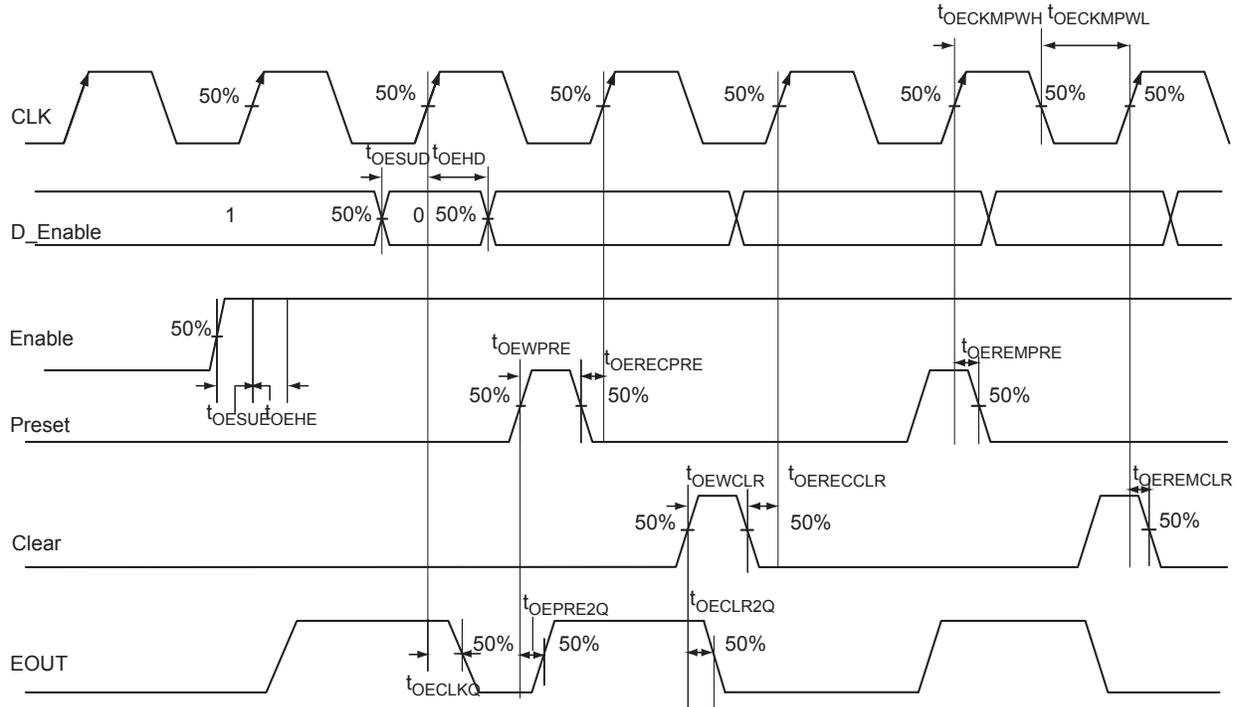
Figure 2-18 • Output Enable Register Timing Diagram
