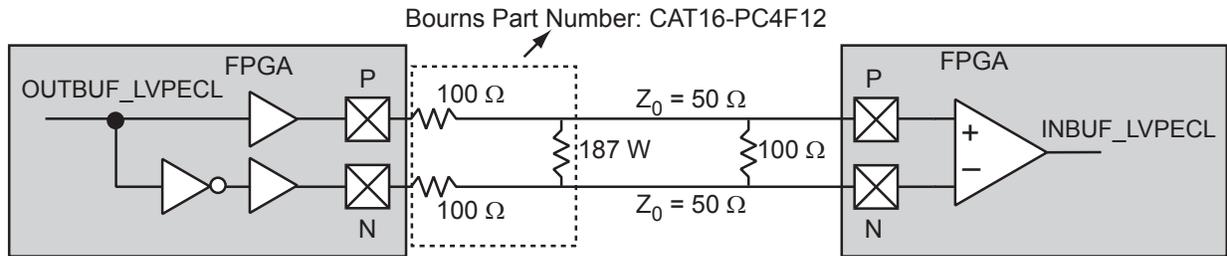
Figure 2-13 • LVPECL Circuit Diagram and Board-Level Implementation
