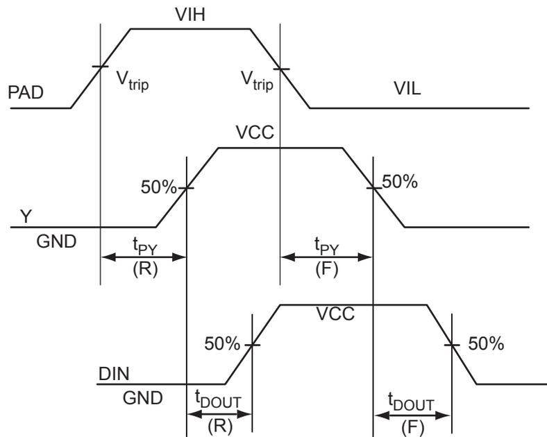
**Figure 2-3 • Input Buffer Timing Model and Delays (example)**
