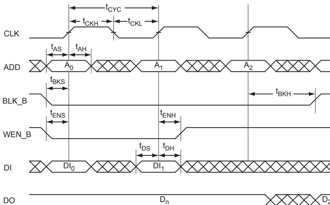
**Figure 2-32 • RAM Write, Output Retained (WMODE = 0)**
