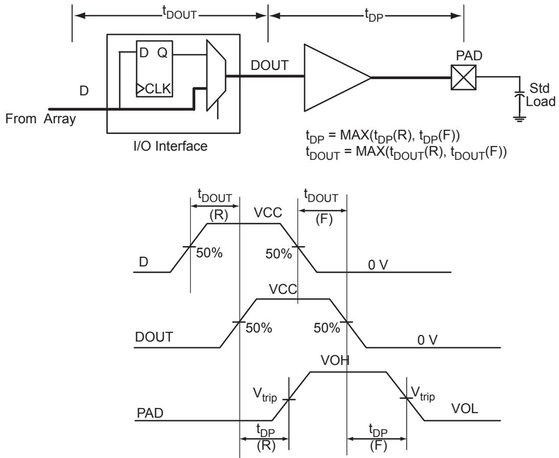
Figure 2-4 • Output Buffer Model and Delays (example)
