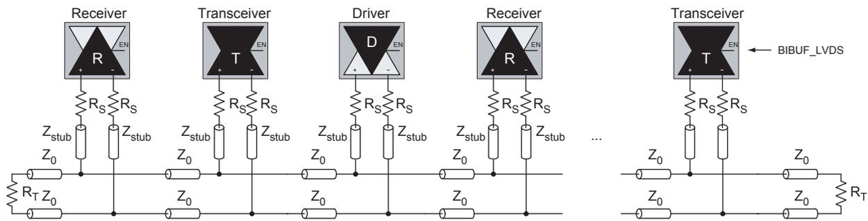
Figure 2-12 • B-LVDS/M-LVDS Multipoint Application Using LVDS I/O Buffers
