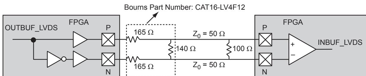
**Figure 2-11 • LVDS Circuit Diagram and Board-Level Implementation**
