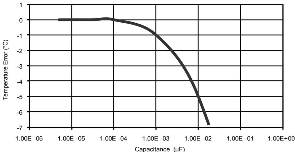
**Figure 2-41 • Temperature Error Versus External Capacitance**
