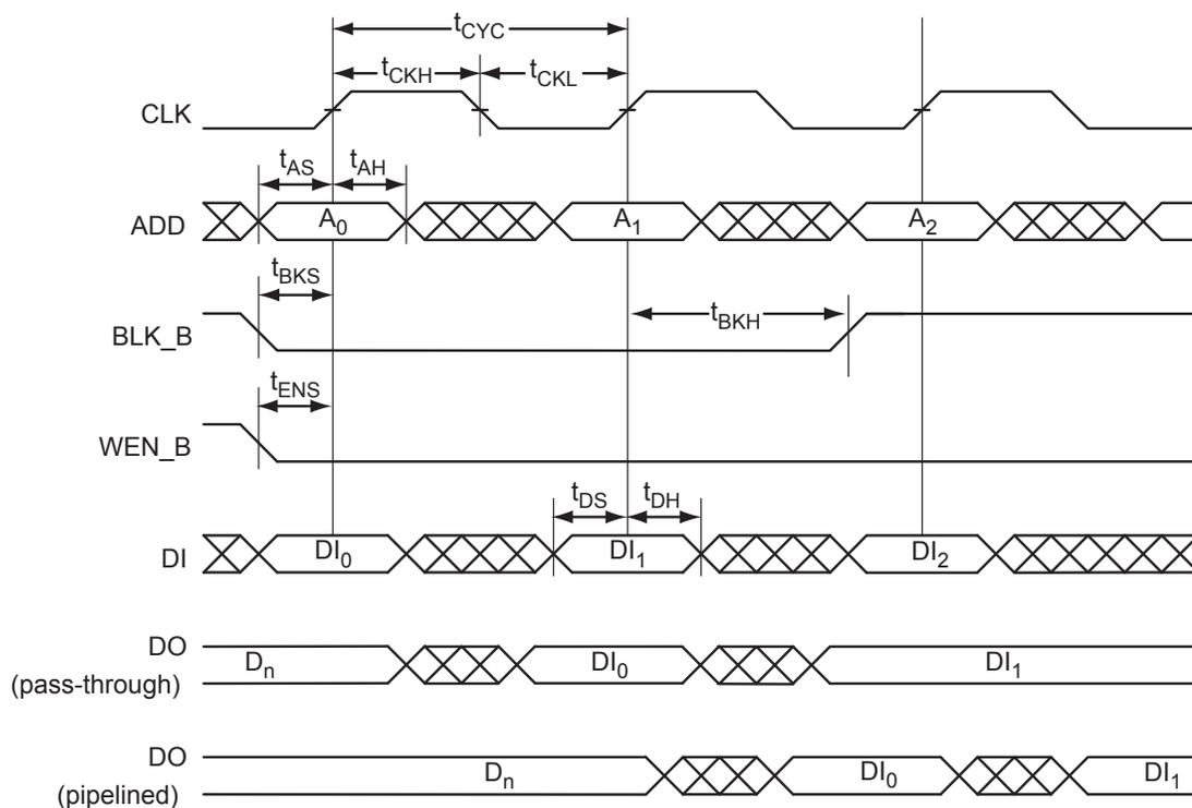
**Figure 2-33 • RAM Write, Output as Write Data (WMODE = 1)**
