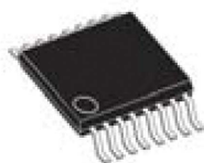
HTSSOP16 ( R_{TH} = 40\text{ }^{\circ}\text{C/W} )
