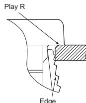
When processing the panel, be sure that the Play R is on the switch operation side.
