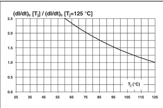
Figure 12. Relative variation of static dV/dt immunity versus junction temperature<sup>(1)</sup>
