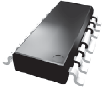
S3 Package Modified 16 Pin SOIC
