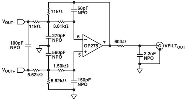
Figure 13. Suggested Output Filter Schematic
