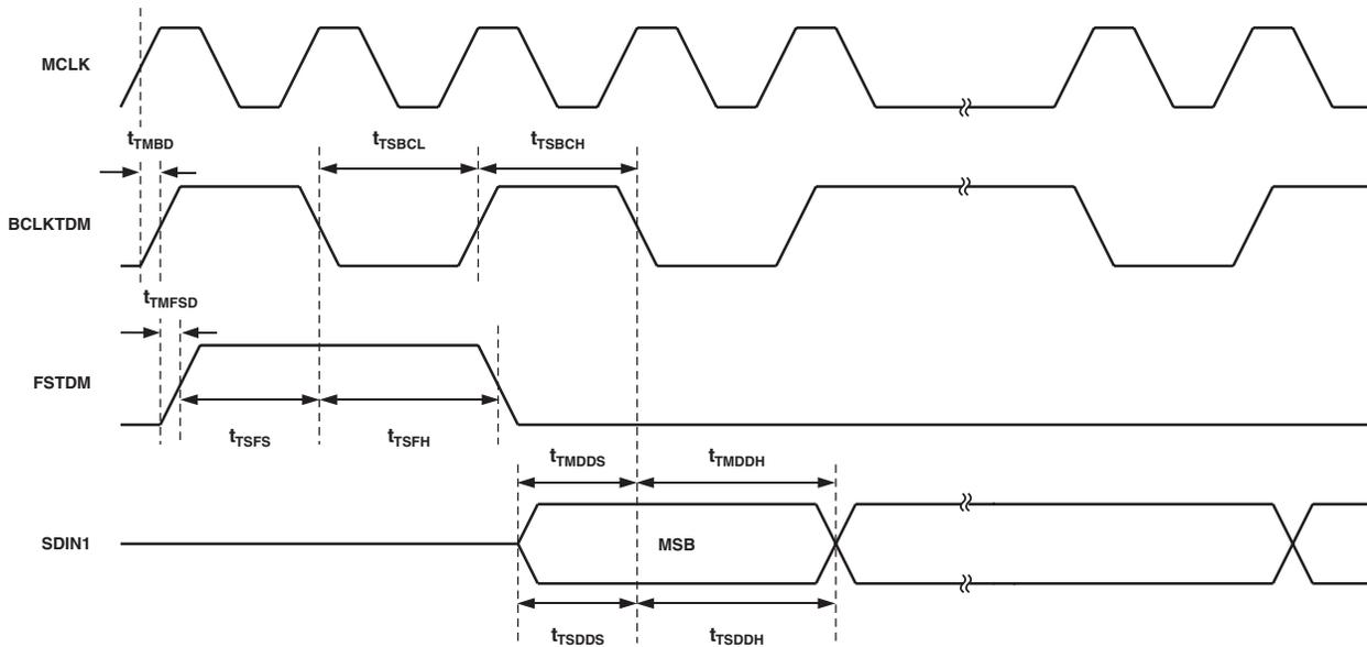
Figure 4. TDM Master and Slave Mode Timing
