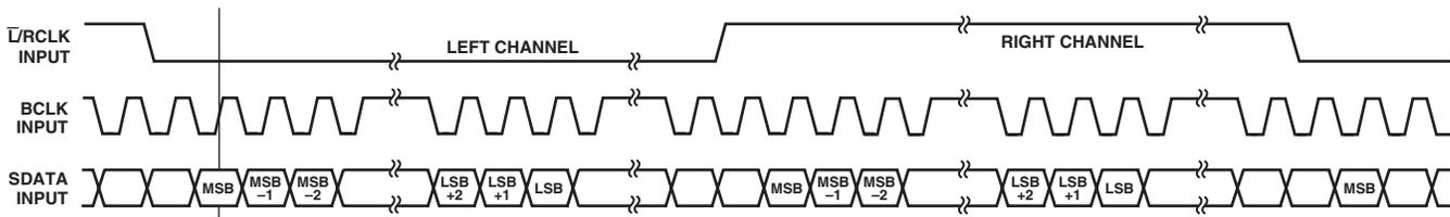
Figure 6. I<sup>2</sup>S Timing Diagram
