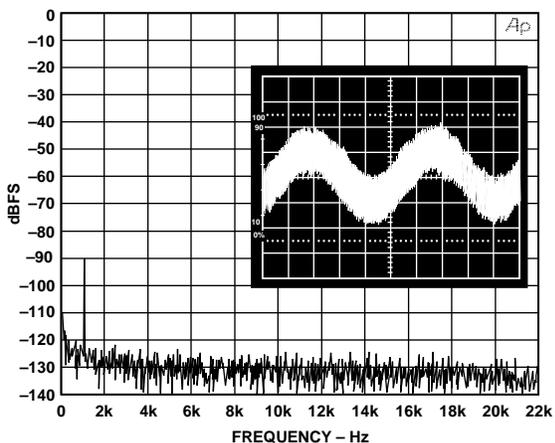
Figure 30. 1 kHz Tone at -90 dBFS (16K-Point FFT) Including Time Domain Plot Bandlimited to 22 kHz
