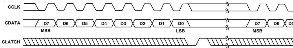
Figure 7. Serial Control Port Timing
