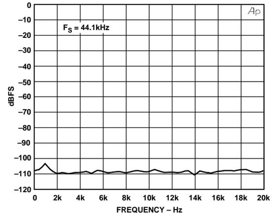
Figure 29. Channel Separation vs. Frequency at -0.5 dBFS
