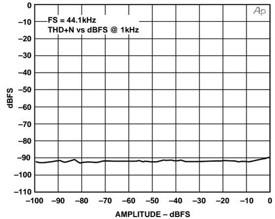
Figure 27. THD+N vs. Amplitude at 1 kHz
