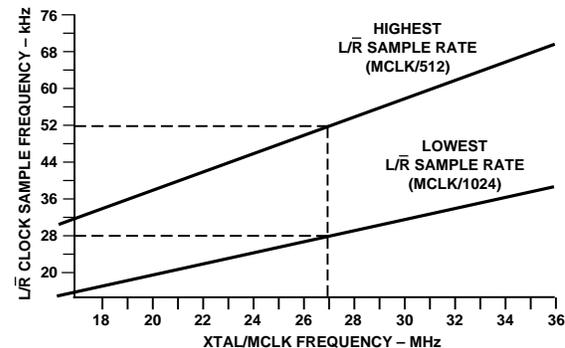
Figure 10. MCLK Frequency vs. L/R Clock Frequency
