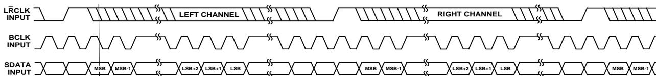
Figure 5. Left-Justified DSP Serial Port Style Mode
