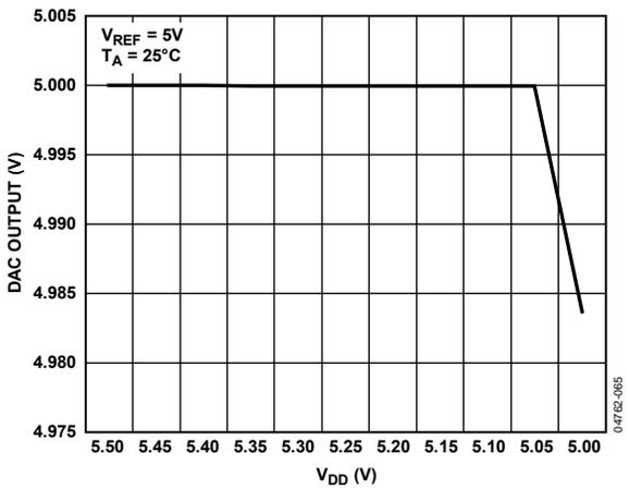
Figure 29. Typical Output Voltage vs. Supply Voltage
