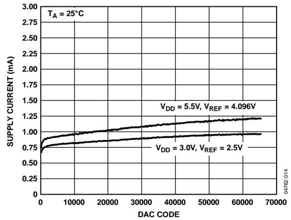
Figure 14. Supply Current vs. Digital Input Code
