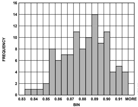
Figure 23.  $I_{DD}$  Histogram @  $V_{DD} = 3V$
