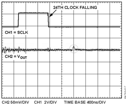
Figure 17. Digital-to-Analog Glitch Impulse; See Figure 21
