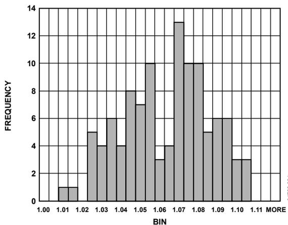
Figure 24.  $I_{DD}$  Histogram @  $V_{DD} = 5V$
