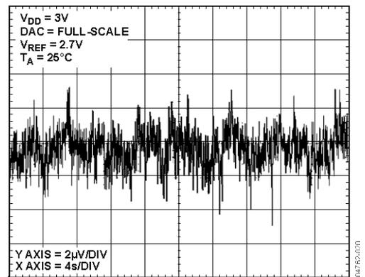
Figure 20. 0.1 Hz to 10 Hz Noise Plot
