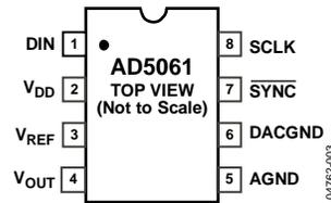
Figure 3. Pin Configuration
