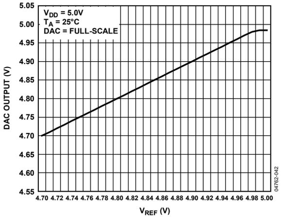
Figure 28. Typical Output Voltage vs. Reference Voltage
