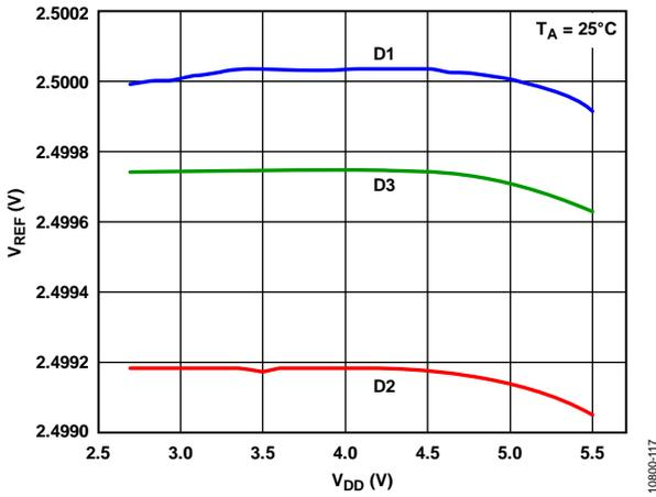
Figure 14. Internal Reference Voltage vs. Supply Voltage
