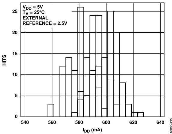
Figure 27. I<sub>DD</sub> Histogram with External Reference, 5 V
