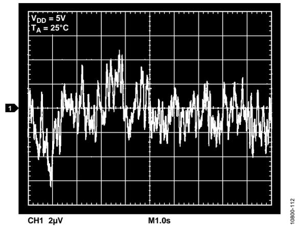
Figure 12. Internal Reference Noise, 0.1 Hz to 10 Hz
