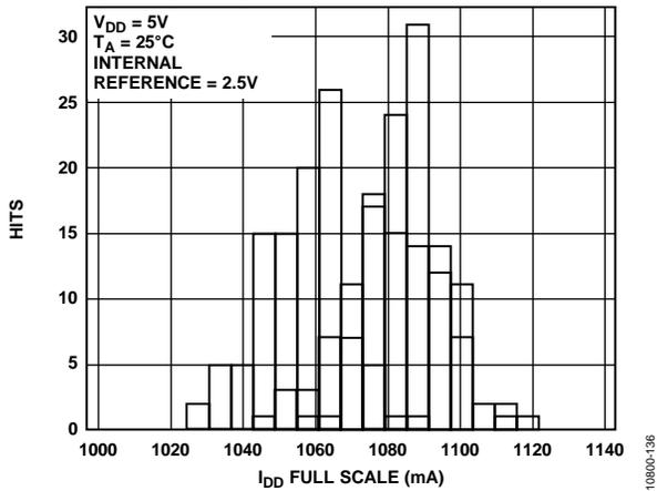
Figure 28. I<sub>DD</sub> Histogram with Internal Reference, V<sub>REF</sub> = 2.5 V, Gain = 2
