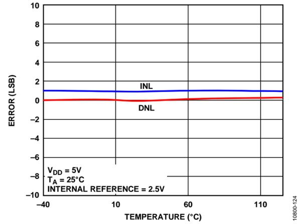
Figure 17. INL Error and DNL Error vs. Temperature
