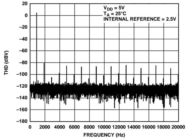
Figure 41. Total Harmonic Distortion @ 1 kHz
