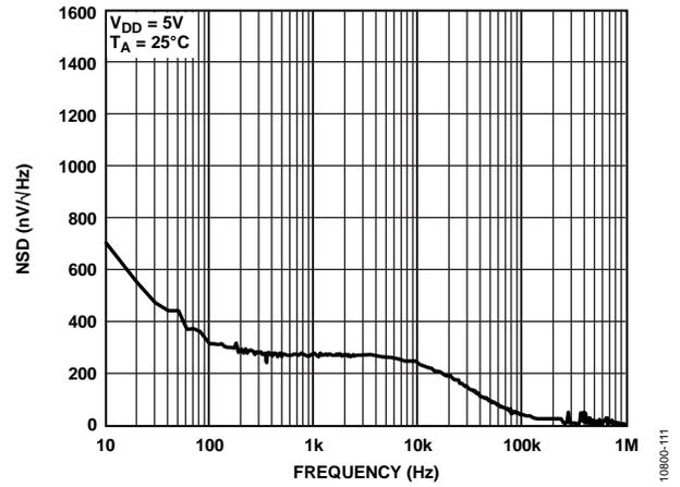
Figure 11. Internal Reference Noise Spectral Density vs. Frequency
