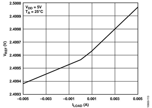
Figure 13. Internal Reference Voltage vs. Load Current
