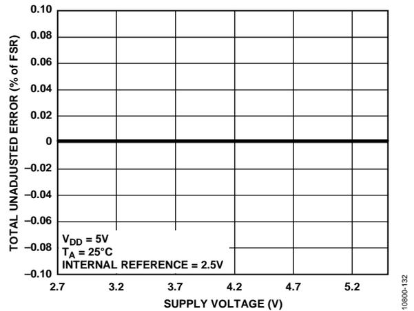
Figure 25. TUE vs. Supply Voltage, Gain = 1
