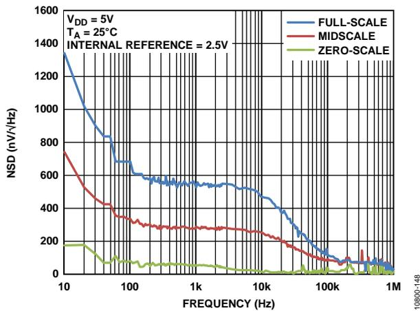
Figure 40. Noise Spectral Density
