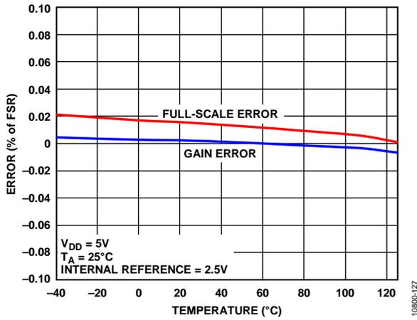
Figure 20. Gain Error and Full-Scale Error vs. Temperature
