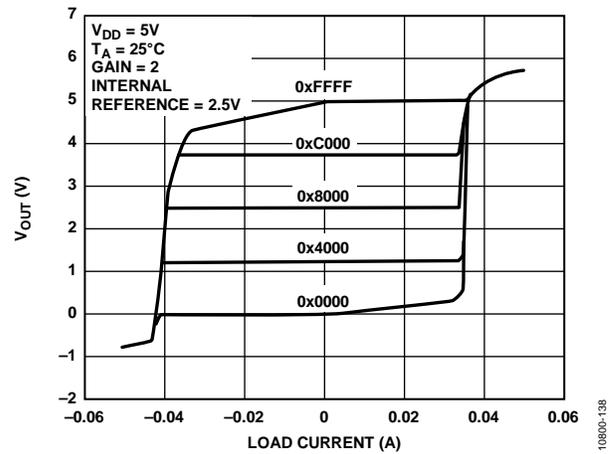
Figure 30. Source and Sink Capability at 5 V
