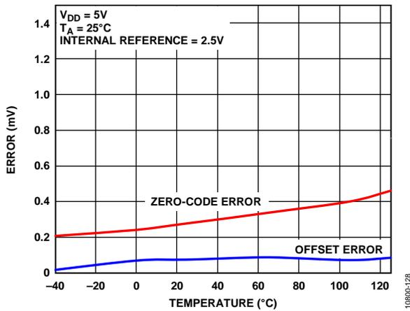
Figure 21. Zero-Code Error and Offset Error vs. Temperature
