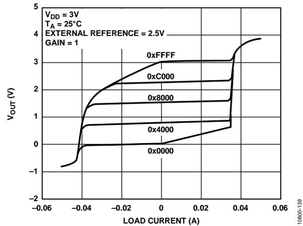
Figure 31. Source and Sink Capability at 3 V
