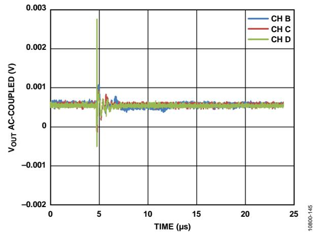
Figure 37. Analog Crosstalk, Channel A
