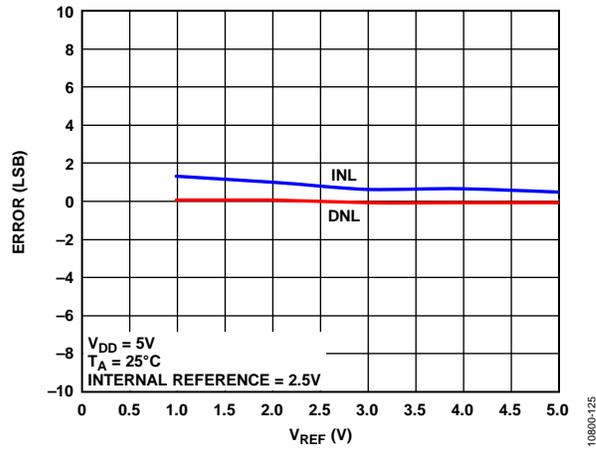
Figure 18. INL Error and DNL Error vs.  $V_{REF}$
