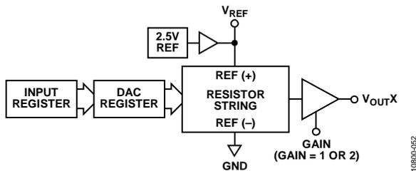
Figure 43. Single DAC Channel Architecture Block Diagram
