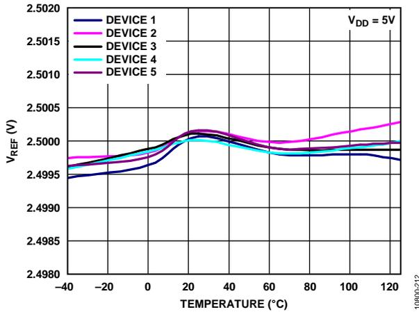
Figure 8. Internal Reference Voltage vs. Temperature (Grade B)
