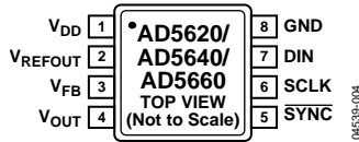
Figure 4. MSOP Pin Configuration
