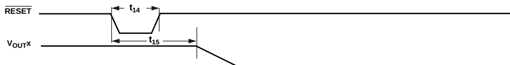
Figure 3. \overline{\text{RESET}} Timing Diagram
