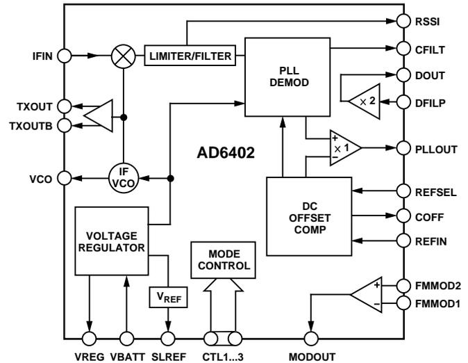
data output. On transmit, it accepts a Gaussian Frequency Shift Keying (GFSK) baseband signal, low-pass filters the signal if required using the on-chip op amp and modulates the IF VCO by varying the bias voltage on an off-chip varactor diode used in the tank circuit.
