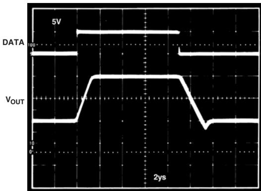
Figure 6. Dynamic Response ( $V_{SS} = -5\text{ V}$ )
