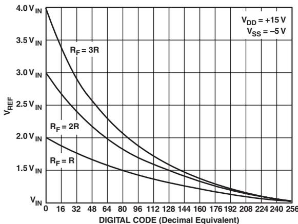
Figure 12. Variation of  $V_{REF}$  with Feedback Configuration
