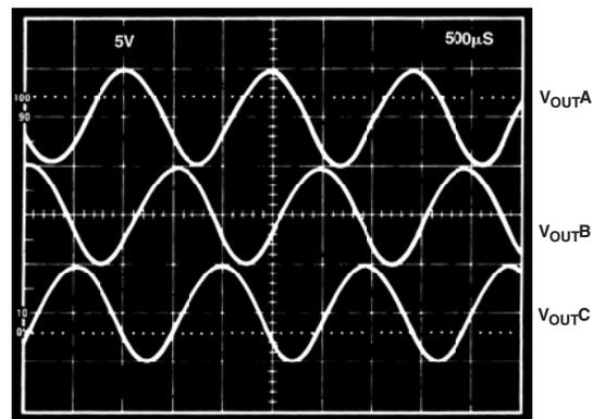
Figure 13. 3-Phase Sine Wave Output
