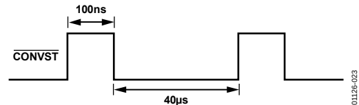
Figure 21. CONVST When Temperature Channel Selected
