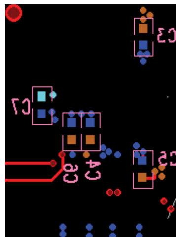
Figure 63. Bottom Layer Decoupling
