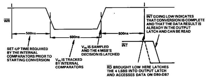
Figure 3. Operating Sequence ( $\overline{WR}$ -RD Mode)
