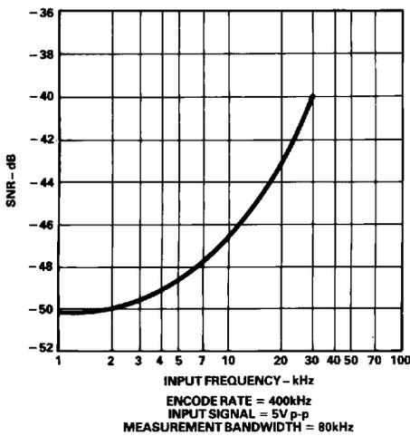
Signal-to-Noise Ratio vs. Input Frequency
