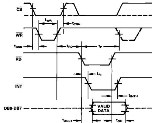
Figure 5b. WR-RD Mode ( $t_{RD} < t_{INTL}$ )
