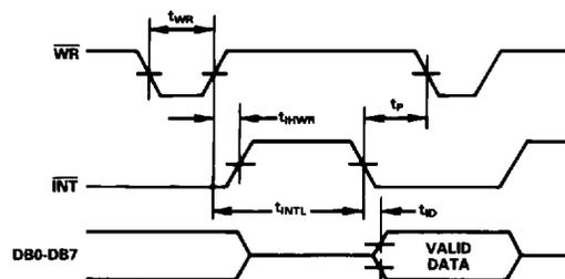
Figure 6. WR-RD Mode Stand-Alone Operation,  $\overline{CS} = \overline{RD} = 0$
