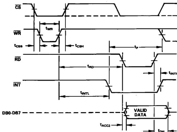
Figure 5a. WR-RD Mode ( $t_{RD} > t_{INTL}$ )
