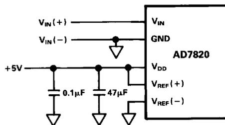
Figure 7a. Power Supply as Reference
