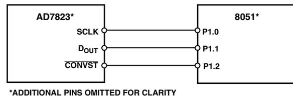
Figure 20. Interfacing to the 8051 Using I/O Ports
