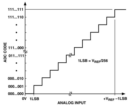
Figure 11. Transfer Characteristic
