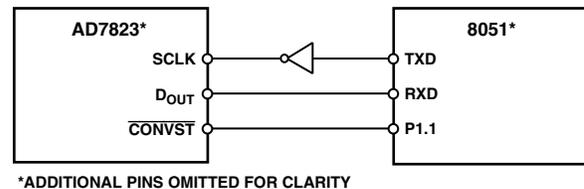
Figure 19. Interfacing to the 8051 Serial Port
