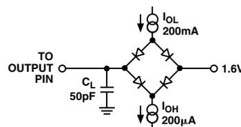
Figure 1. Load Circuit for Digital Output Timing Specifications
