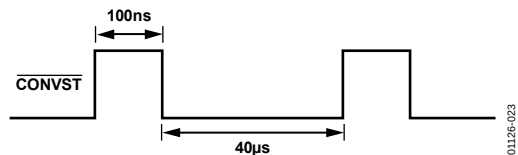
Figure 21. \overline{\text{CONVST}} When Temperature Channel Selected
