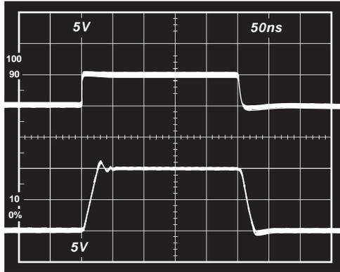
TPC 31. Noninverting Large Signal Pulse Response;
