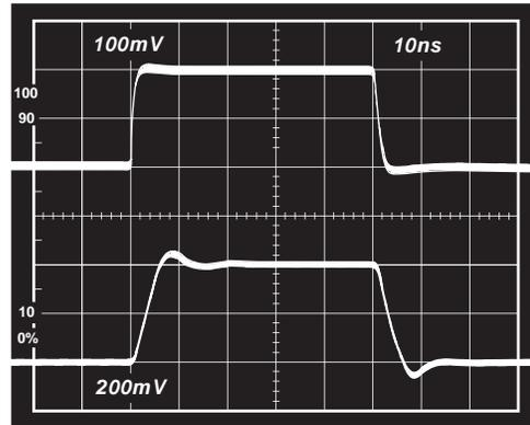
TPC 33. Noninverting Small Signal Pulse Response;
