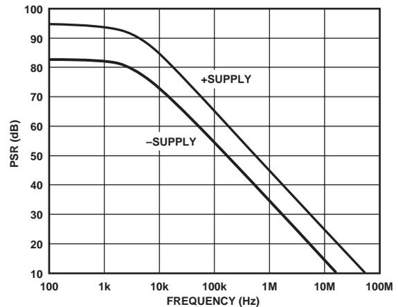
TPC 12. Power Supply Rejection vs. Frequency
