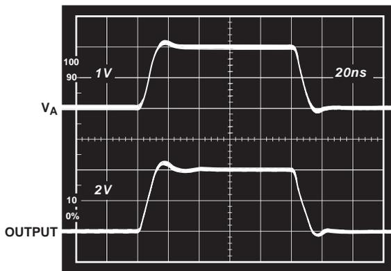
Figure 10. Performance of Line Receiver,  $R_L = 150 \Omega$ ,  $G = +2$
