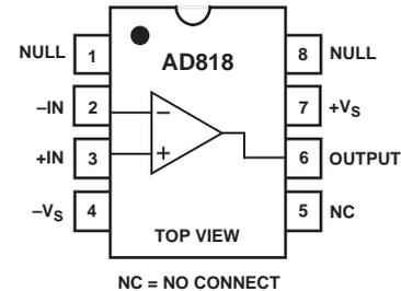
any video application. The 130 MHz 3 dB bandwidth (G = +2) and 500 V/ms slew rate make the AD818 useful in many high speed applications including video monitors, CATV, color copiers, image scanners, and fax machines.
