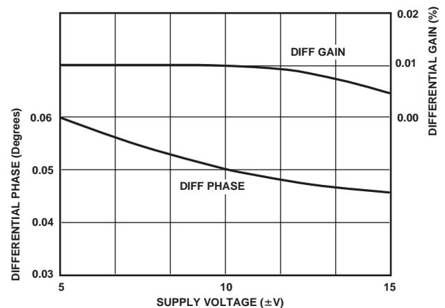
Figure 2. Differential Gain and Phase vs. Supply
