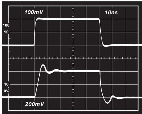
TPC 32. Noninverting Small Signal Pulse Response;
