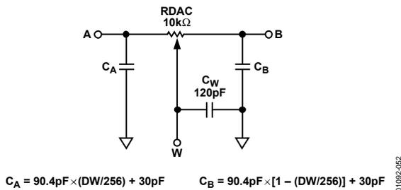
Figure 53. RDAC Circuit Simulation Model for RDAC = 10 kΩ
