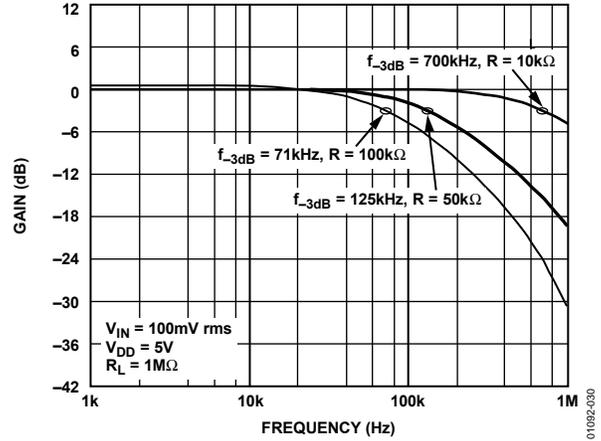
Figure 30. -3 dB Bandwidths
