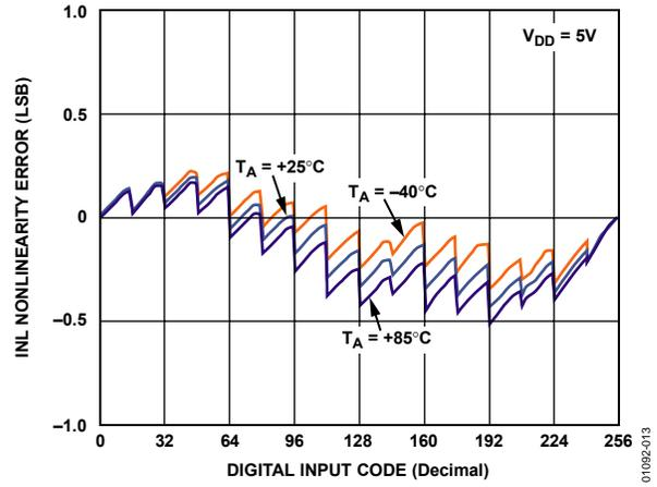
Figure 13. Potentiometer Divider Nonlinearity Error vs. Code
