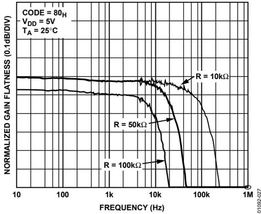
Figure 27. Normalized Gain Flatness vs. Frequency
