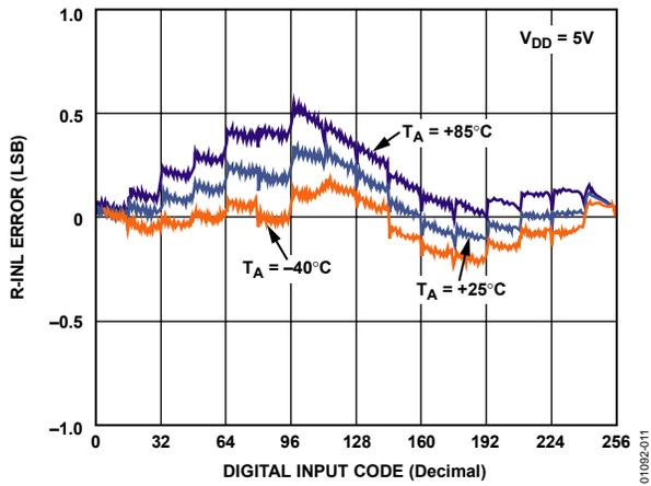
Figure 11. Resistance Step Position Nonlinearity Error vs. Code
