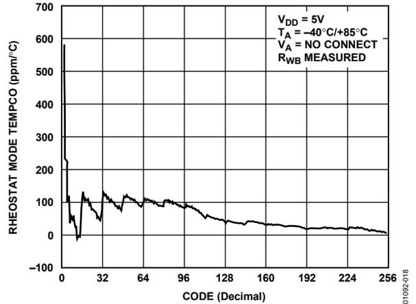
Figure 18.  $\Delta R_{WB}/\Delta T$  Rheostat Mode Tempco
