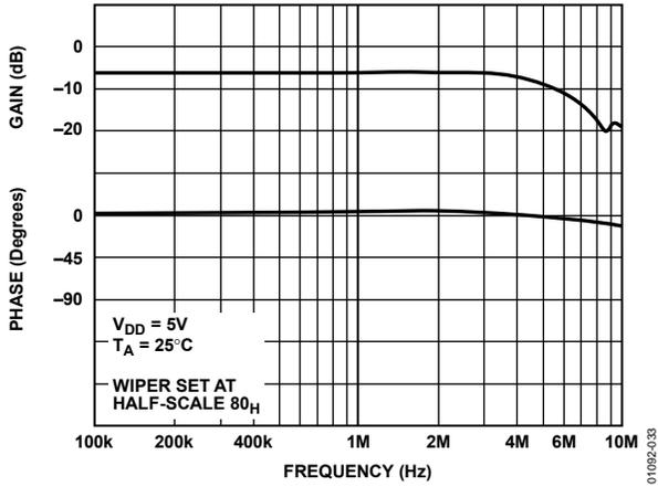
Figure 33. 1 k $\Omega$  Gain and Phase vs. Frequency
