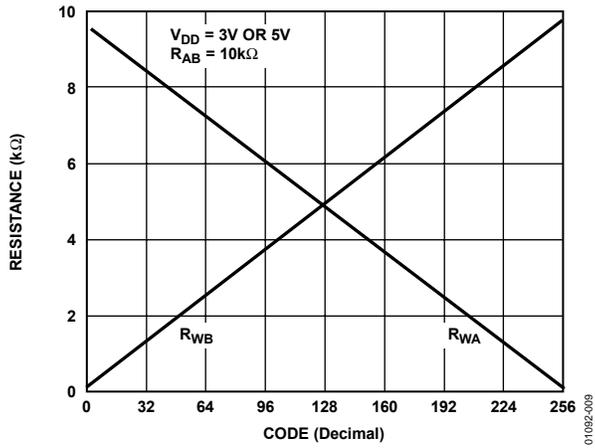
Figure 9. Wiper to End Terminal Resistance vs. Code
