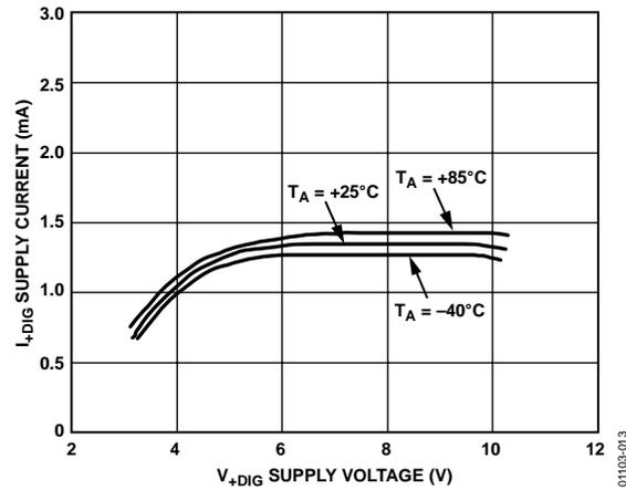
Figure 13.  $I_{+DIG}$  Supply Current/Comparator vs.  $V_{+DIG}$  Supply Voltage
