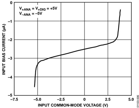
Figure 6. Input Bias Current vs. Input Common-Mode Voltage
