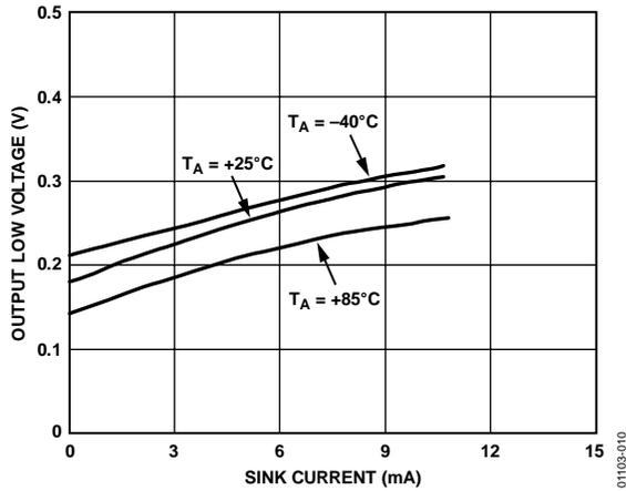
Figure 10. Output Low Voltage,  $V_{OL}$  vs. Sink Current
