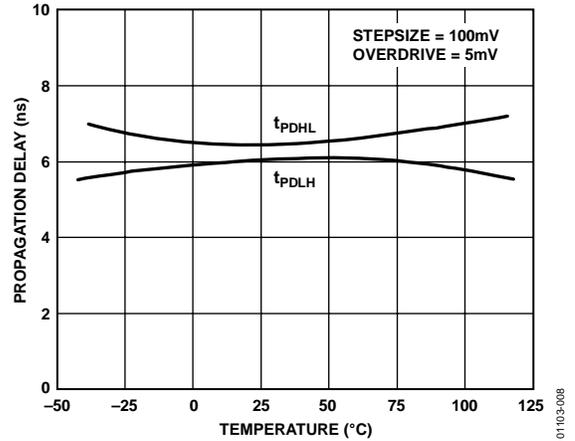
Figure 8. Propagation Delay,  $t_{PDHL}/t_{PDLH}$  vs. Temperature
