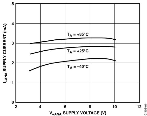
Figure 11.  $I_{+ANA}$  Supply Current/Comparator vs.  $V_{+ANA}$  Supply Voltage
