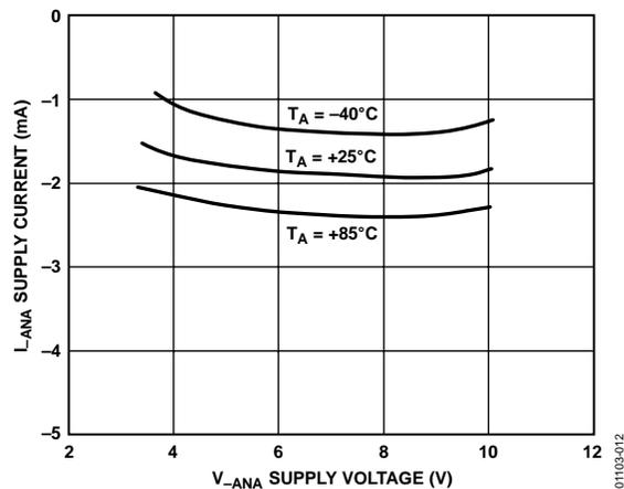
Figure 12.  $I_{-ANA}$  Supply Current/Comparator vs.  $V_{-ANA}$  Supply Voltage
