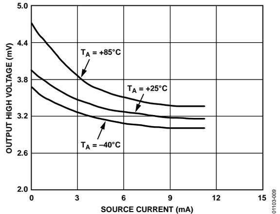
Figure 9. Output High Voltage,  $V_{OH}$  vs. Source Current
