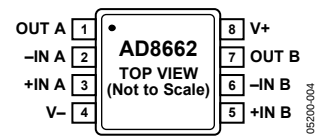
Figure 4. AD8662, 8-Lead MSOP (RM-8)
