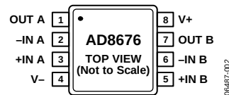
Figure 2. 8-Lead MSOP (RM-8)
