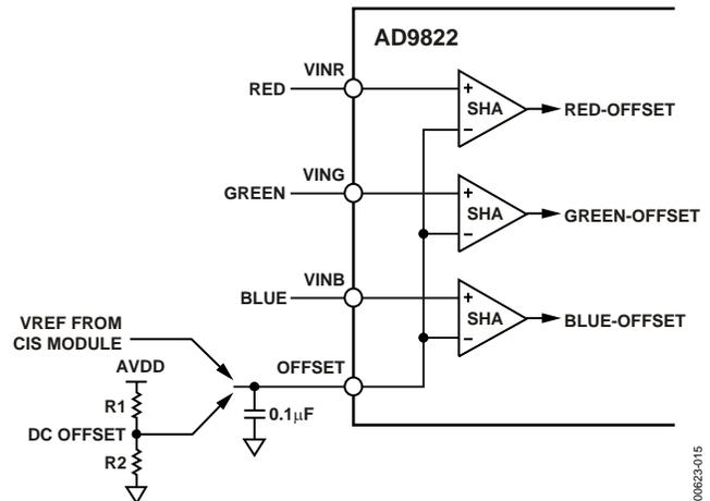
Figure 14. SHA Mode Used with External DC Offset
