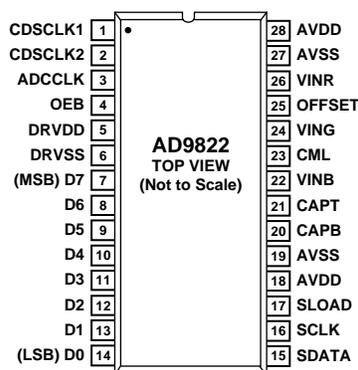
Figure 2. Pin Configuration
