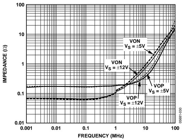
Figure 21. Single-Ended Output Impedance vs. Frequency and Supplies
