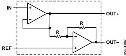
Figure 41. Functional Diagram
