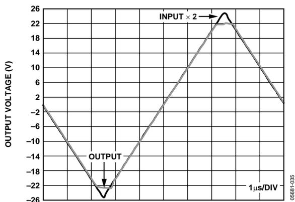
Figure 32. Input Overdrive Recovery,  $V_S = \pm 12V$
