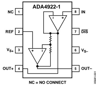
Figure 4. Pin Configuration
