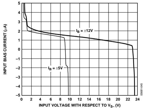
Figure 38. Input Bias Current vs. Input Voltage
