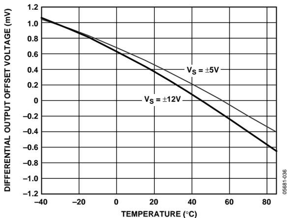
Figure 30. Differential Output Offset Voltage vs. Temperature
