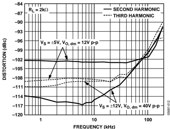
Figure 17. Harmonic Distortion for Various Power Supplies
