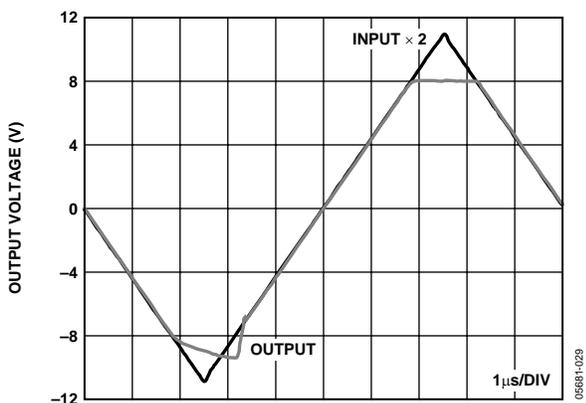
Figure 29. Input Overdrive Recovery,  $V_S = \pm 5V$
