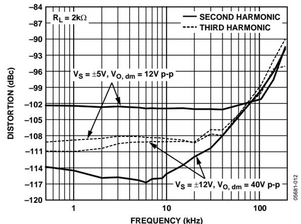
Figure 2. Harmonic Distortion for Various Power Supplies
